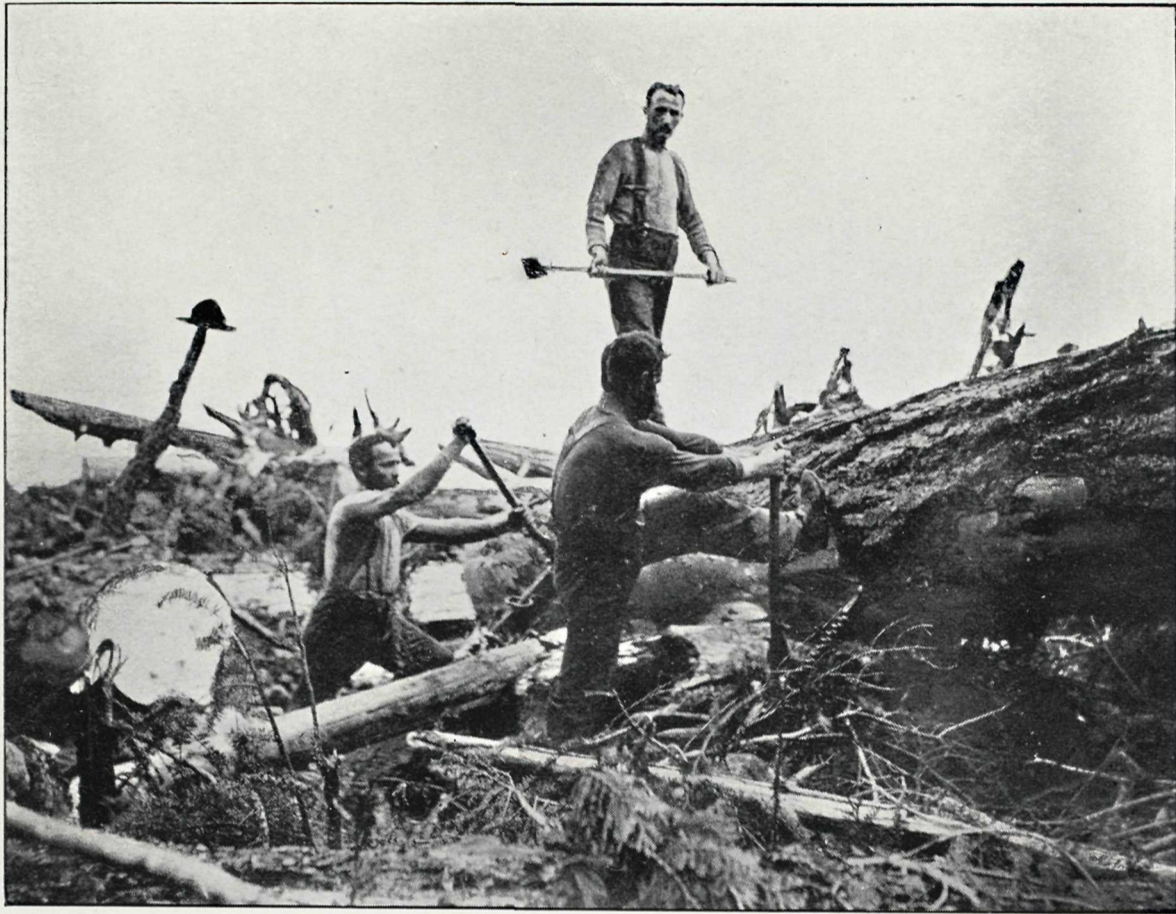
HANDLOGGERS COAXING A LOG : ROLLING IT OVER WITH SCREWS AND BARKING IT.
